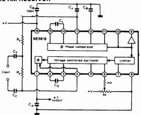
It is possible to construct a simple a.m. receiver using a single off-the-shelf phase-locked-loop integrated circuit, together with a few external components. A major advantage of this approach is that no tuning coils are needed. Sensitivity can be improved with the addition of a wide-band r.f. amplifier front end, but it is important that the input of the phase-locked-loop should not exceed 0.5V r.m.s.
